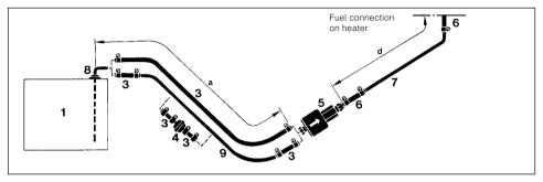
2. If difficulties arise in installing the rising tank connection, the supply line can be tapped.
