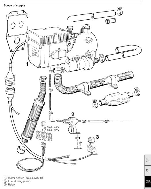
Parts without a Fig. No. are contained in the universal installation kit.
