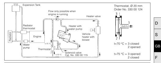
3. Heater in coolant line between engine and heat exchanger of vehicle, with non-return valve installed parallel. No thermostat.
