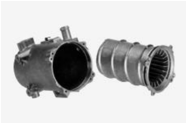
11 Heat exchanger dismantled
