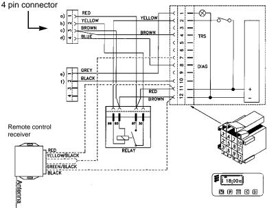
This eg.shows the remote receiver terminated directly to heater, terminations can also take place at the harness connectors. See descriptions above.
